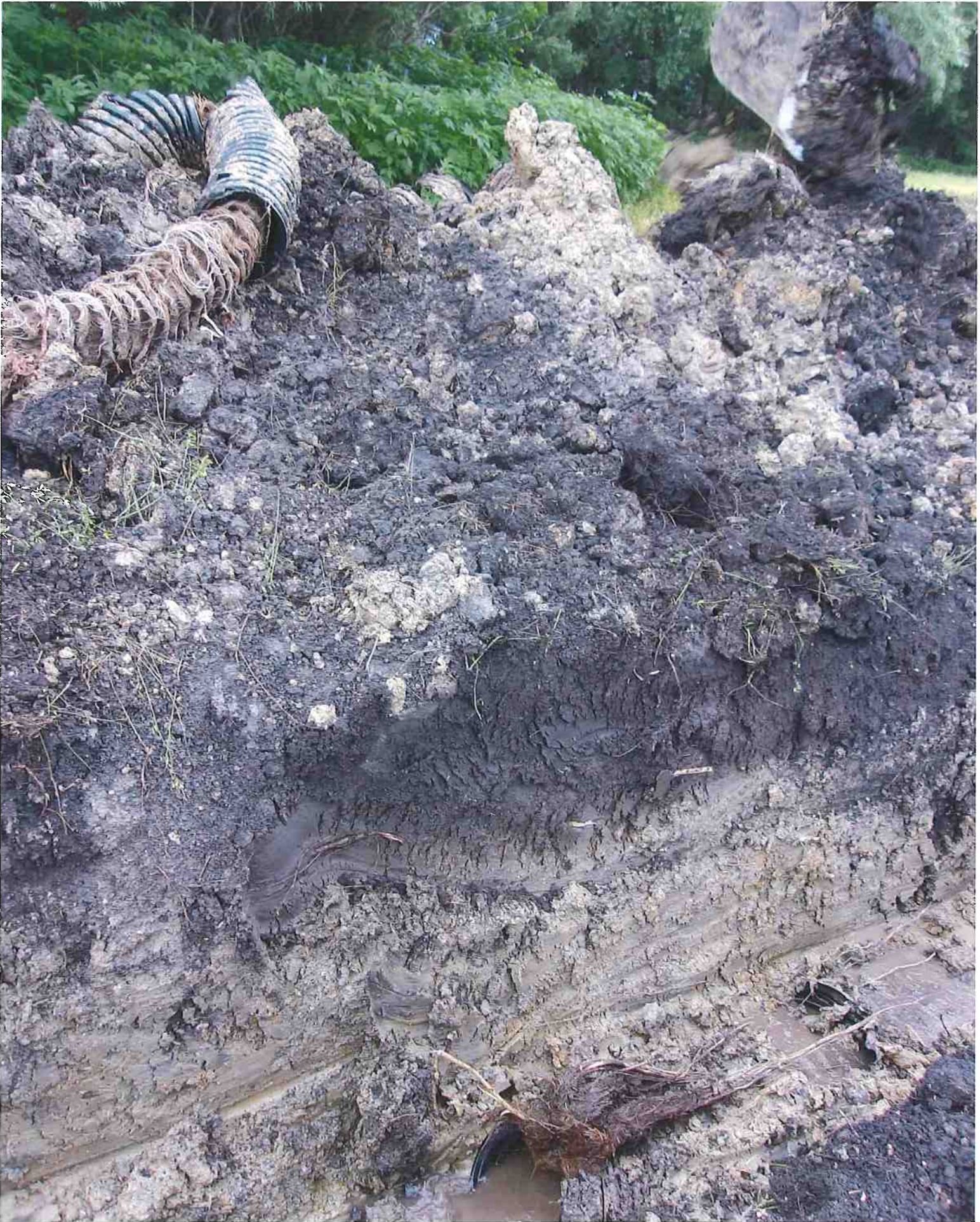
ROOTS GROWING THRU NON PERF. 12" P.E. TUBE
